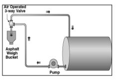
Asphalt scales or "weigh buckets" need to be calibrated to make sure they weigh accurately. This typically involves hanging known weights on the device to make sure the scale instrument is recording the correct weight.
