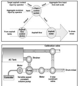
Obviously, for the asphalt content to be correct, the belt scales need to be properly calibrated so they represent accurate flow over all the production rates the plant will run, and the asphalt meter needs to be properly calibrated over the rate which the plant will run. Calibrating over these different speed ranges is a very important point.
