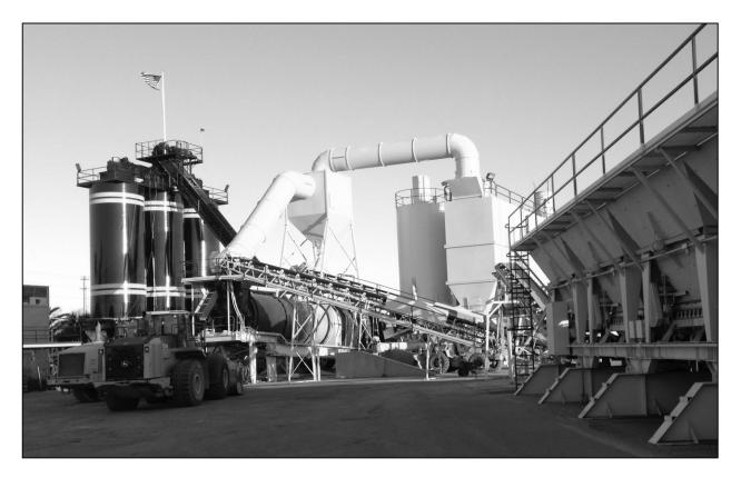
A key thing to remember and focus on when trouble-shooting plant operations is to remember that the asphalt plant (HMA/WMA Facility) is simply a drying, heating, and blending machine.
