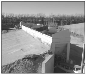
3. The individual aggregate gradations in the stockpiles / being loaded into the feed bins
