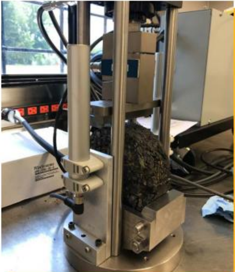
Image Source: FHWA Load Frame performing Ideal-RT
