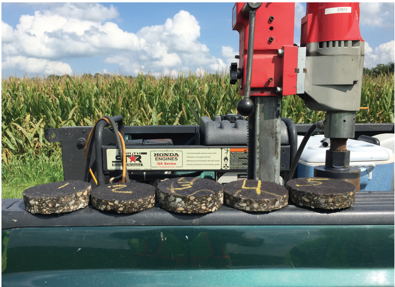
Pavement cores from 2016 Thinlay project in Darke County, Ohio.
